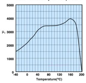
Measured on a 17/10/6mm toroid at 10kHz.
